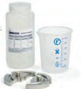
Newtonian, and they are available as either silicone or oil. Silicone fluids are less temperature sensitive than oil fluids. Note: Brookfield recommends that all fluids be replaced annually
